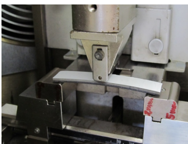
Figure 2 – NOK: Specimen curved upwards
