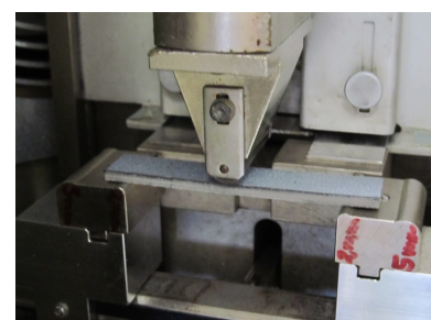
Figure 4 – NOK: Test tool presses onto the wrong side of the specimen
