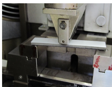
Figure 3 – NOK: Specimen at an angle on the support
